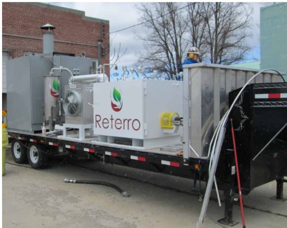
Reterro Mobile EDU with Thermal Oxidizer
